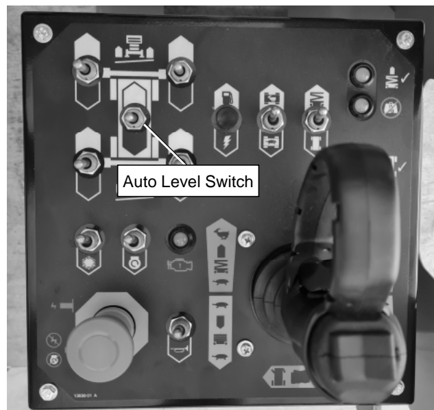
Figure 8.9 – Auto Level Switch
