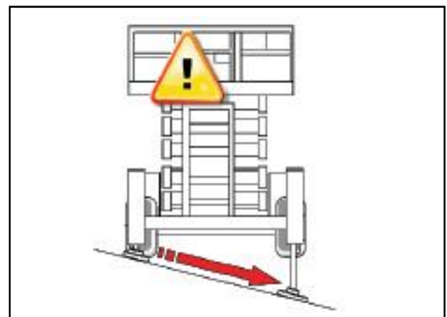
Figure 8.13 – Machine On Slope
