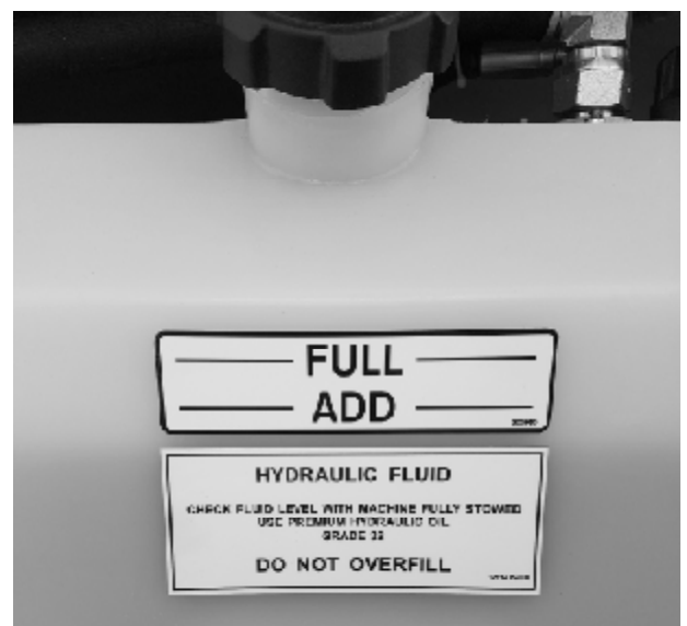
Figure 5.3 Hydraulic Oil Tank
